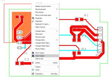
When using poured copper remember you shouldn't use Delete but should always use Clear Copper. Copper Pour Areas can be modified at any time and the area re-poured using the option from the shortcut menu. If you wish to completely remove the copper and area, you must use Clear Copper first and then delete the area afterwards using the Delete key.
