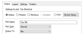
The **Options** button and **Device Setup** button allow you to change the settings of the selected plotter type. For example, changing from RS-274-D to 274-X format for Gerber.
