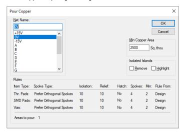
Using the Thermal Pads check box and the Spokes settings, the style of who the copper is connected to pads can be defined.
