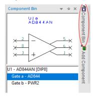
Our Op-Amp (U1) is shown in the Bin as two gates (Gate a & Gate b). Click on Gate a under the word U1 - AD844AN {DIP8} to see a preview of the symbol above it.
