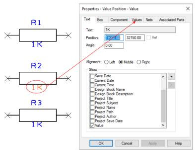
The **Value** field shows the current 1K value and is already highlighted blue. Simply click the **Edit** button or double-click the blue highlighted field to edit the value required. Type in  $\bf 11K$ .
