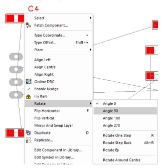
For our design, no mirroring (Flip) will be required. The placement and overall connection lengths could be improved by rotating some of the components. If you feel you would like the practice placing components, select a component and click **R** to rotate it. Component names can be rotated back to be a readable direction separately using the same pick and rotate method.
