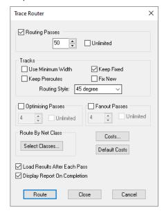
Simply click the Route button at the bottom of the dialog to start the router. This small design will easily route 100%.
