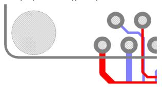
To access this option, go to the Settings menu, Preferences dialog, Display tab. Options are available at the bottom left hand side of the dialog for Cross-Hath Drill Holes with an option to Only When Drilled Out.
