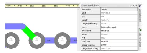
To enable the Properties Bar, click on the View menu. Dockable Bars, and click Properties Bar. Alternatively, right click on the right-hand bar and select **Properties** as shown in the illustration to the right.
