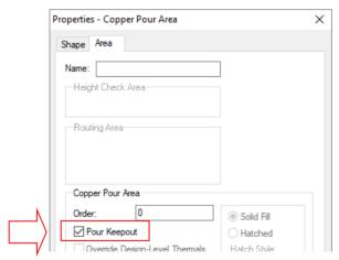
When the Pour Keepout area is added to the design, copper is avoided when poured.
