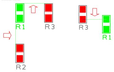
Options are available on the Settings, Preferences, Schematic Interaction/PCB Interaction, Dynamic Align. The settings are dependent on the design environment you are in, therefore allowing you to control the items that will be aligned to and control the Snap Tolerance in both the SCM and PCB. This option can also be enabled from the **Context** menu, when moving an item, right click, and select Use Dynamic Align.
