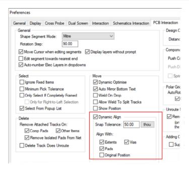
When aligning an item, you can choose to enable the **Dynamic Align** option to align with an item's Extents, a Pad, Via, the item's original position or Text (only text items will align with another text item).
